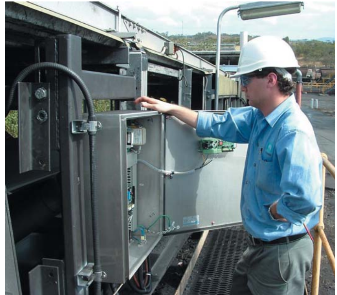
Tarek Kazzaz commissioning the LFM Bowen Moisture Analyser at Dalrymple Bay, Queensland
